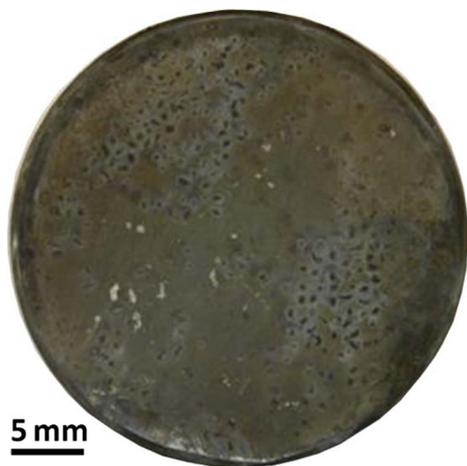
**FIGURE 7.** Electrochemical sample with corrosion product layer after removal of the sand particles for the experiment with inhibitor CI(29) at 100 ppm.
